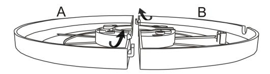
Thread the power cord through the hole made by the 2 base parts and then place the base on the bottom of the main body of the heater and secure with the 4 screws provided.
